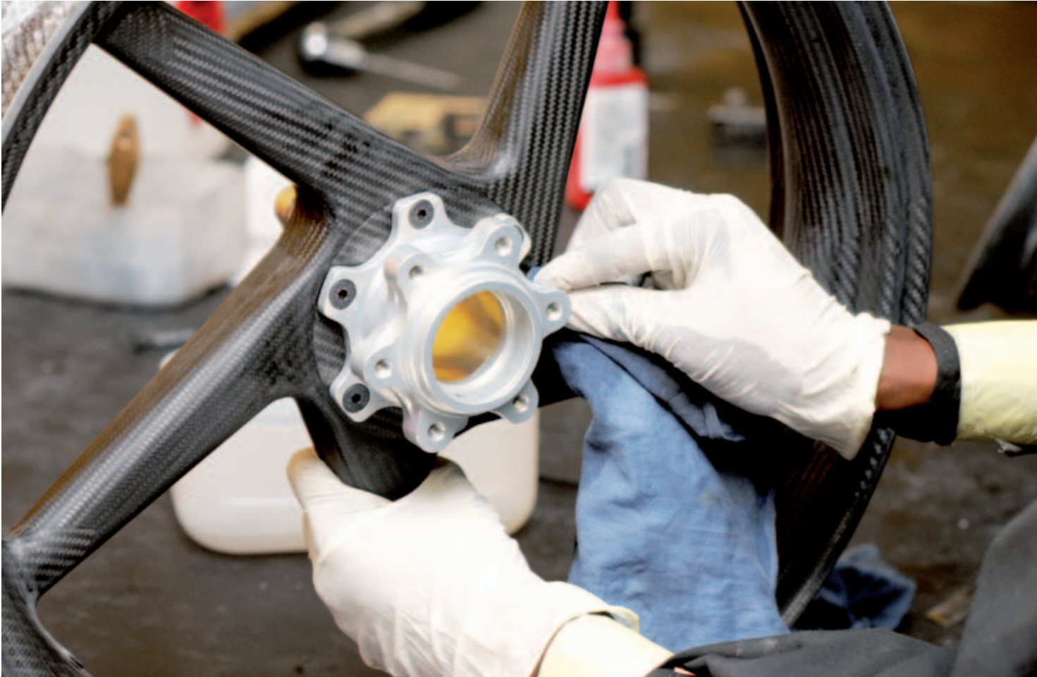
Each BST wheel design is comprised of between 130 and 180 different individual carbon components, each of which must first be CNC laser-cut from the roll of pre-preg material, then individually numbered. ///
