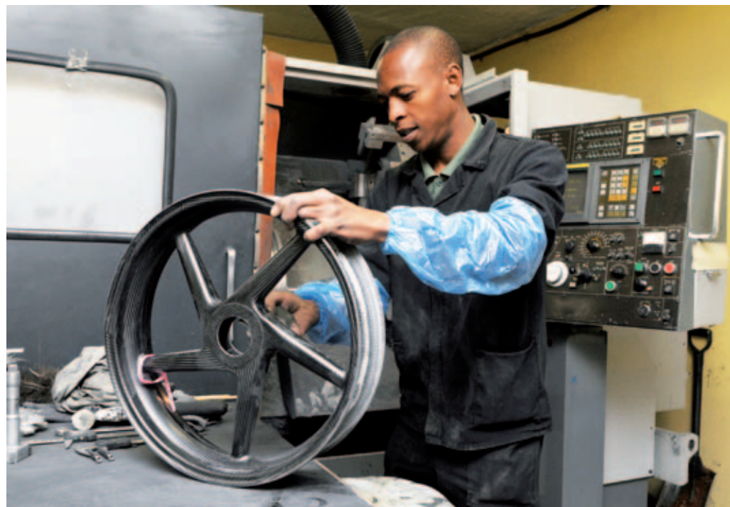
Each wheel is initially built in two halves which are then joined together in a strong single unit before baking. ///
