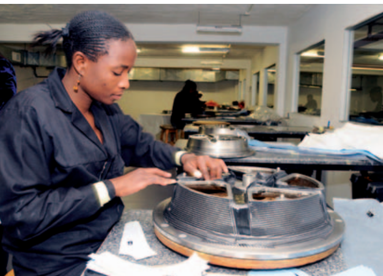
The wheels are built by BST's team of skilled assemblers - around half of them women - working in two separate clean rooms with positive air pressure to not compromise the integrity of the finished product. ///
